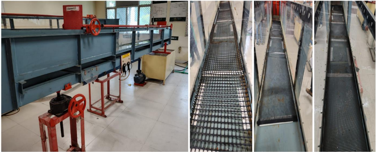
Fig-2:- Roughness coefficient testing done in open channel flume
